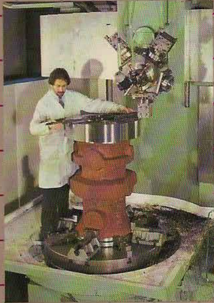
1,250mm Elevating Rail Series 'S' CNC Machining valve body.
