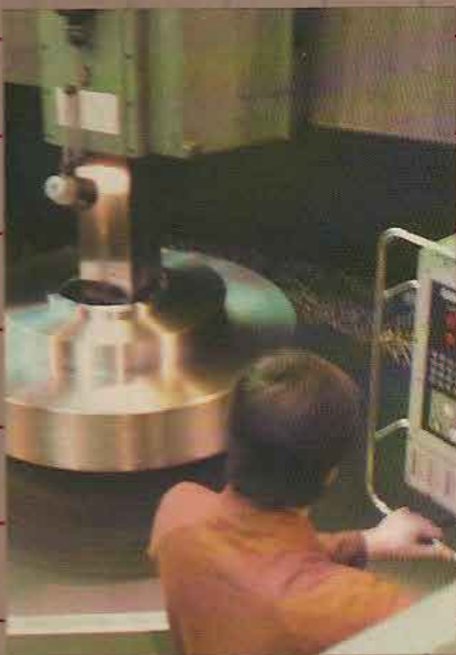
120" DCS CNC machining a pump component.
