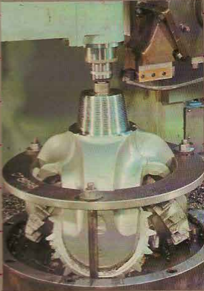
1,000mm Fixed Rail Series 'S' CNC machining Taper threads of 26" diameter rock bit for the oil industry.
